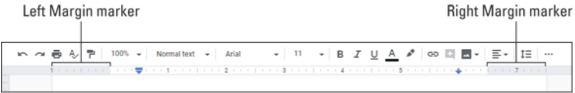
FIGURE 7-10: Drag the margin markers to adjust the left and right margins.
